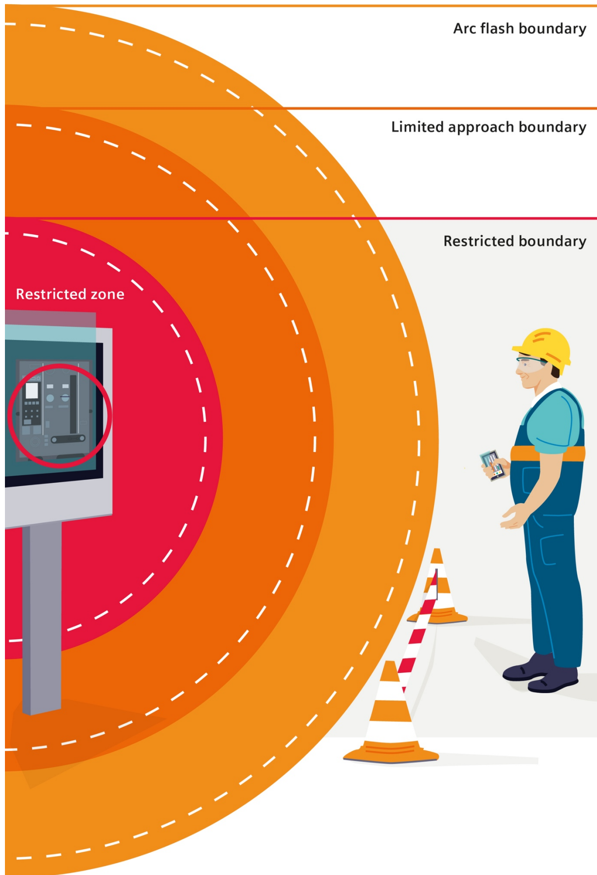
Figure 3: Protection zones for working on live parts
